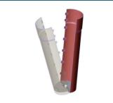
1. Clip two halves together 2. Push base disc into place, once halves assembled
